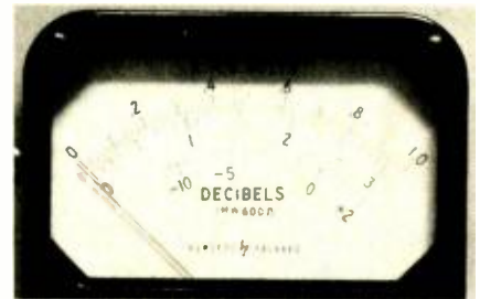
VOLTMETER WITH dB SCALE referenced to 0.775 volt. See Solving The dB Mystery for more data. . . . turn to page 65
