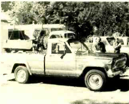
BIG SUR FIRE-FIGHTING VEHICLE , with slip-on in place and CB mast visible above the cab. Besides having their own tanks, the units can pump from an external water supply, such as a pond or stream.
