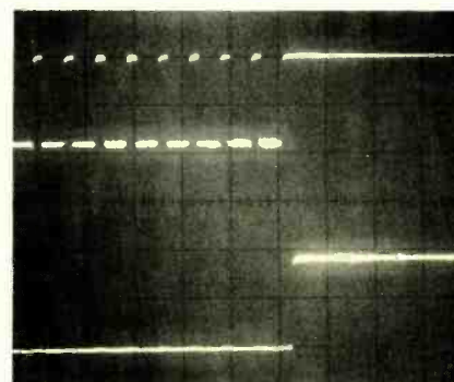
FIG. 5—SINGLE-DIGIT PULSE TRAIN is obtained by expanding the trace shown in Fig. 4.
